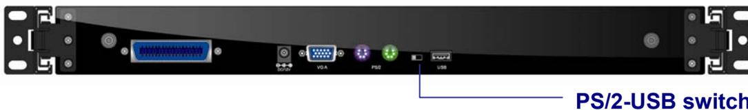
Figure 4-1. Back view of ComboXCAT console drawer
