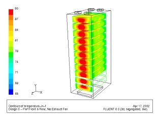
**Figure 1 shows** air flow for an enclosure with top vents and perforated front and rear doors. Air exhausted from individual servers is 90F+.
