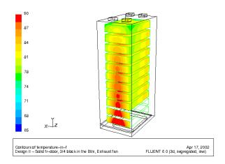
**Figure 2** shows an improvement in cooling efficiency using a non-perforated front on the enclosure. The solid front door reduces the amount of computer room ambient air pulled into the enclosure, increasing the amount of air drawn up from the raised floor cooling system.
