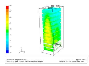
**Figure 3 shows** a dramatic reduction in server exhaust air temperatures using the Delphi ECS Enclosure Blower, indicating much greater cooling efficiency from the redirected air flow in the enclosure.
