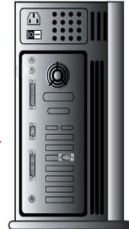
4. Plug the **SINGLE** blue HDB15 connector to anyone of Sylphit-Duo DSK ports numbered 1 through 8 (or 16).
