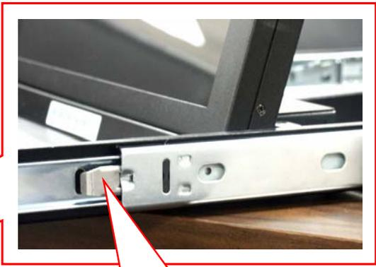
Press the lever to unlock
