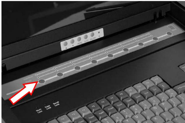
**A solid green "Power" LED** indicates that the server connected to the associated port is powered up.
