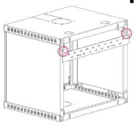
After securing the hanging bracket to the wall, lift the cabinet and hang it on the two points going through the square clearance holes on the back of the cabinet.
